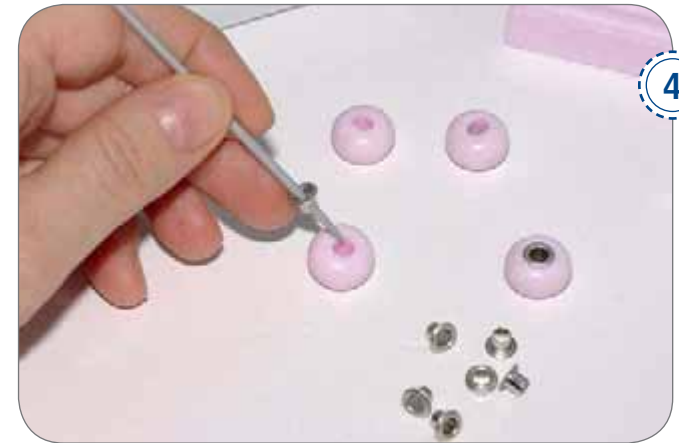
Use the knitting needle to place the eyelets exactly into the holes and press on gently with your finger.
